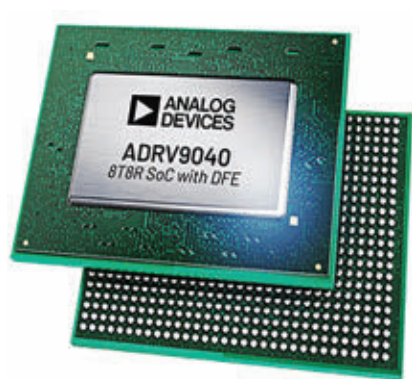
2. Though this is a larger SoC, coming in a 27- × 20-mm, 736-ball BGA housing, the transceiver has eight receivers and transmitters for 650 to 6000 MHz. Analog Devices
