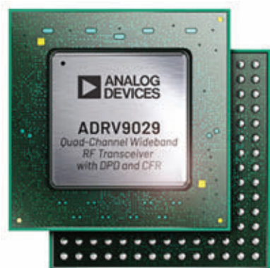
1. As an example of an SoC, this 75- to 6000-MHz agile transceiver is housed within a 289-ball, CSP_BGA package measuring 14 × 14 mm. Analog Devices
